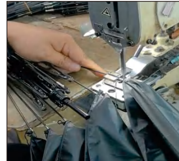
8. 露先と生地縫製 Canopy Stitched to Ribs
